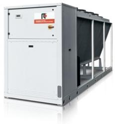
Outdoor unit for the production of chilled water with hermetic rotary Scroll compressors, low-GWP and ozone-friendly refrigerant R454B, axial-flow fans, plate heat exchanger, micro-channel full-aluminum air coils and thermostatic or electronic expansion valve, according to the model. The range is composed by units equipped with two compressors in a single-circuit configuration.
